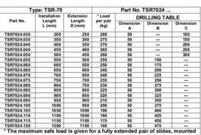
on the major axis, with a load spread uniformly along the inner beam
